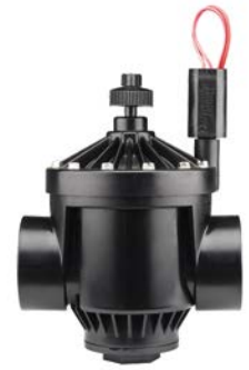
PGV-201 VALVE Inlet diameter: 2" (50 mm) Height: 20 cm Length: 17 cm Width: 13 cm
