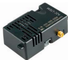
A2C-LTEM Height: 7.6 cm Width: 5.7 cm Depth: 2.5 cm
