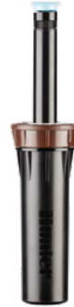
PROS-04-PRS30 Retracted height: 15.5 cm Pop-up height: 10 cm Exposed diameter: 5.7 cm Inlet size: ½"
